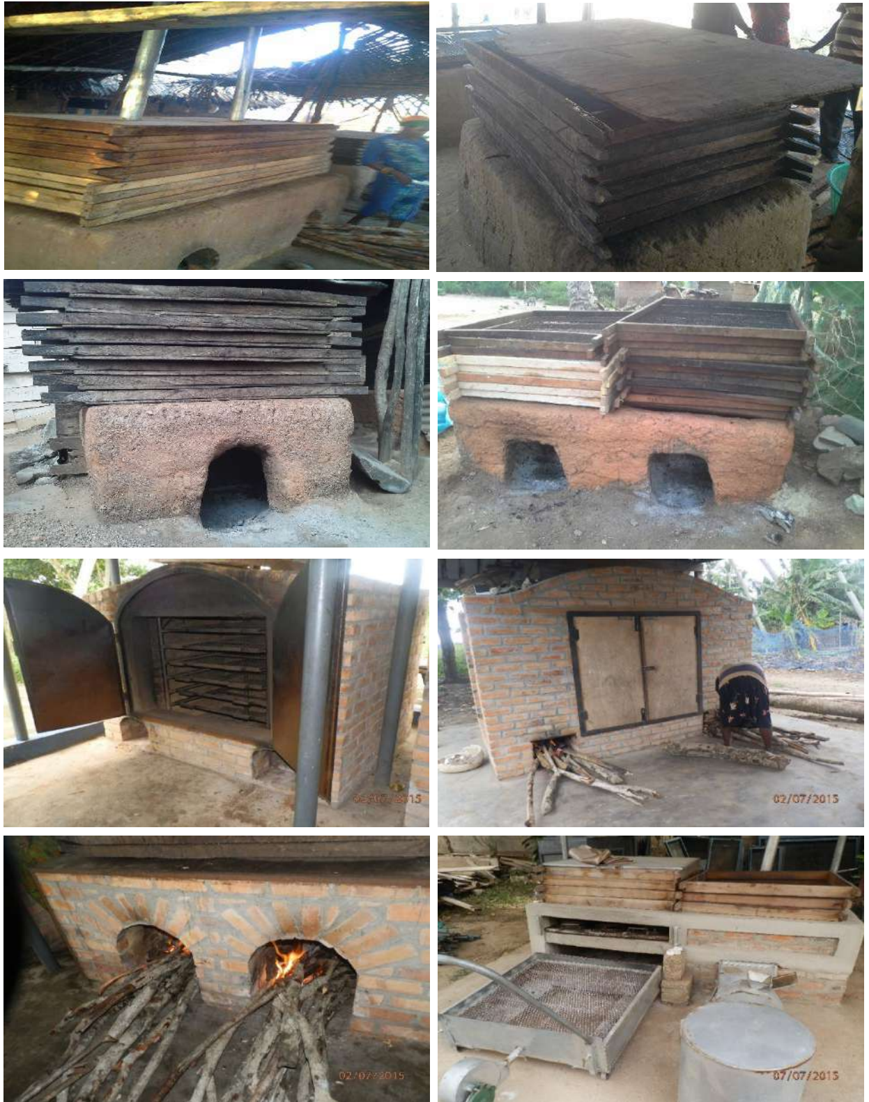
Figure 1 Photograph of testing stoves (a) Morrison, (b) Chorkor-Ada, (c) AWEF, (d) Chorkor-Otuam, (e) KOSMOS Oven, (f) TULLOW Oven, (g) Chorkor KOSMOS and (h) FTT.
