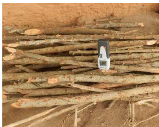
Figure 3: Measurement of woodfuel moisture content
